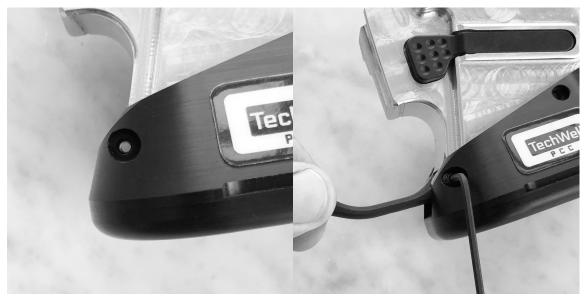
Step 2: Make sure that the front of the Techwell is up and solidly held in place position, then insert the pointy short screws into the front holes. Again, make sure not to strip the threads by turning the screws left at first to make sure that the threads align. Then turn the screws carefully, a bit at a time on each side until they make contact, then just like one turn on each side which should hold the Techwell firmly in place, and you're good to go ....
